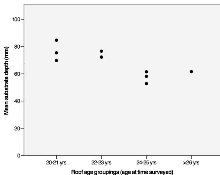
**Figure 2 Mean substrate depth decreases on extensive green roofs over time.**
