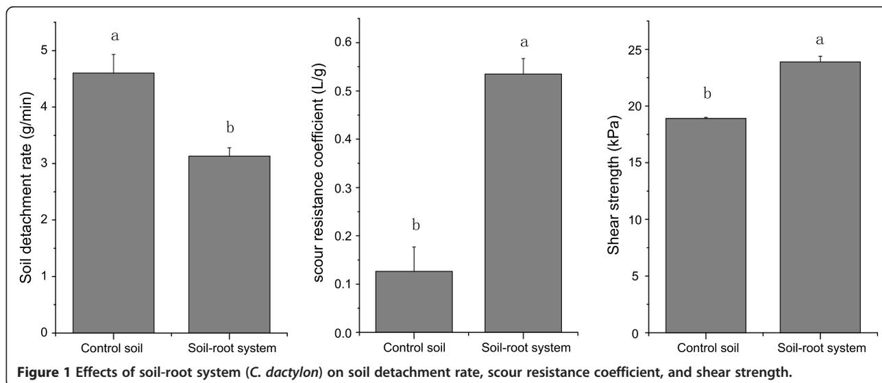
**Figure 1 Effects of soil-root system (*C. dactylon*) on soil detachment rate, scour resistance coefficient, and shear strength.**
